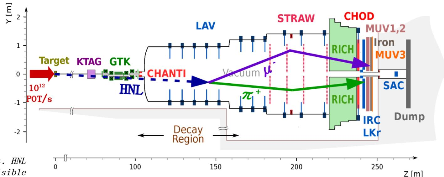
NA62 schematic layout. HNL signal topology is visible
