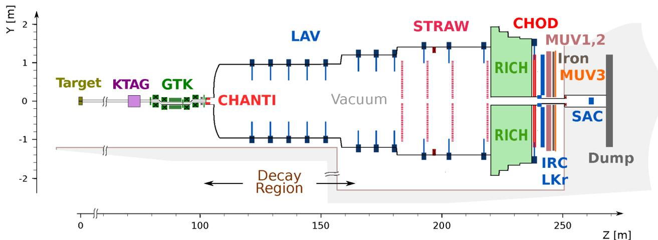
NA62 schematic layout. All detectors are visible
