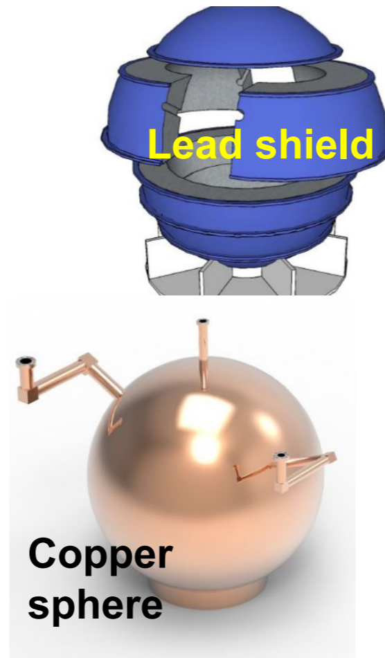
Simulation done with 12mm thick 140cm diam copper sphere full with 99% Ne 1%CH 4 , 11.43 kg of gas
