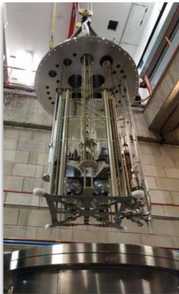
Assembly of TPC into cryostat
