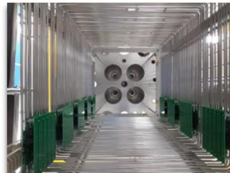
View of voltage dividers / inside TPC
