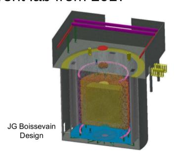
New cavern needed to accommodate AIT-WATCHMAN ( $\sim$ 25m  $\phi$  x  $\sim$ 25m h)
