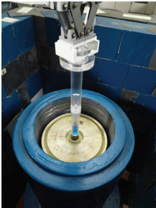
Figure 3. (Left) NPL ionization chamber with ampoule of radioactive material entering the well; (Right) Activity time distribution and half-life fits for the decay of ^{223}\text{Ra} obtained using this ionization chamber [11].
