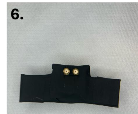
Entire detector wrapped in light-tight tape
