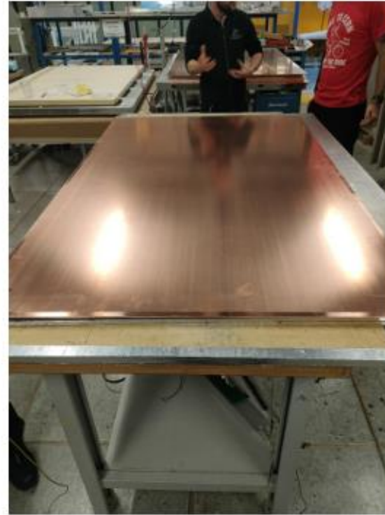
Step3: Put another readout pannel on the top of the gas gap
