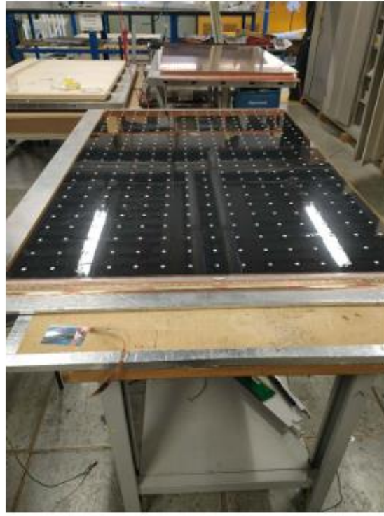
Step2: Put the gas gap on the top of the readout pannel
