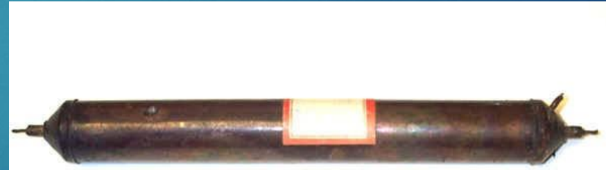
A Geiger-Müller counter built in 1939 and used in the 1947-1950 for cosmic ray studies in balloons and on board B29 aircraft by Robert Millikan et al.
