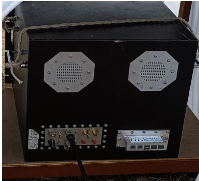
Shielding cage to enclose the Laptop, Spectrum analyzer and the receiver
