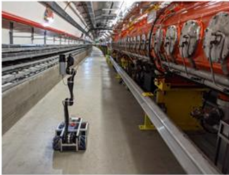
-Left: Mira3 robot used for robotic interventions –Right: Map created using Karto SLAM at Dump area
