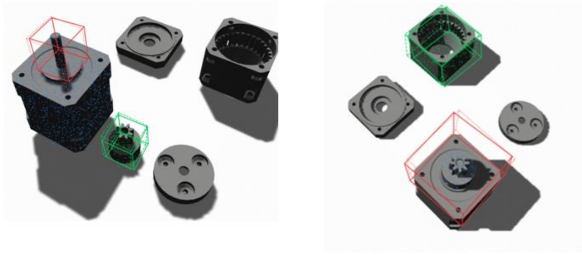
Assembly instance results. Green boxes indicate target-pose estimates and red boxes indicate assembled-target estimates; dashed boxes indicate the corresponding ground-truth poses
