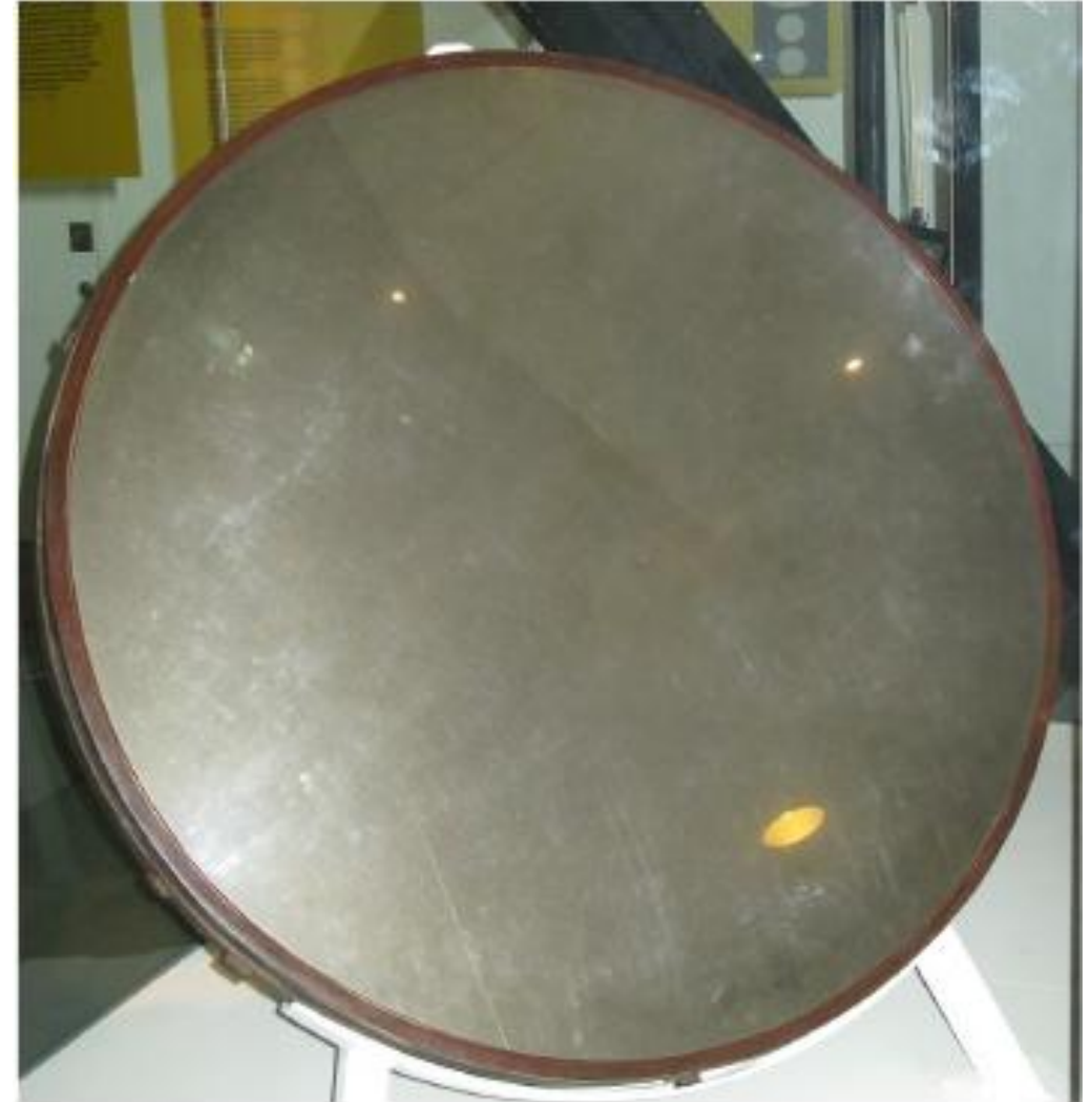
Herschel's 1.2m mirror made of "speculum" (copper and tin) in 1789
