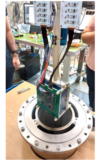
Insertion into cryostat
