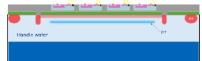
(b) Structured AC-LGAD in SOI wafer
