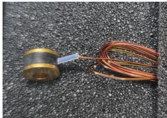
4-wire Cernox M3 mounting Range: RT - 4 K
