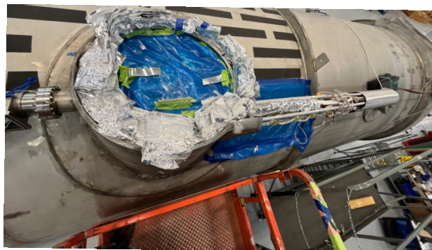
Chimney complete; solenoid ends dry-fit
