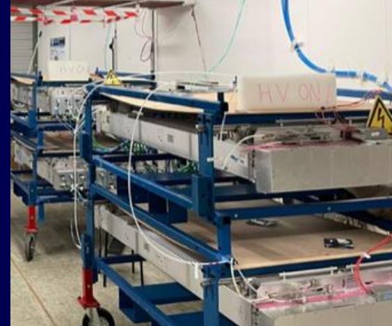
UM Muon Chambers under test at CERN
