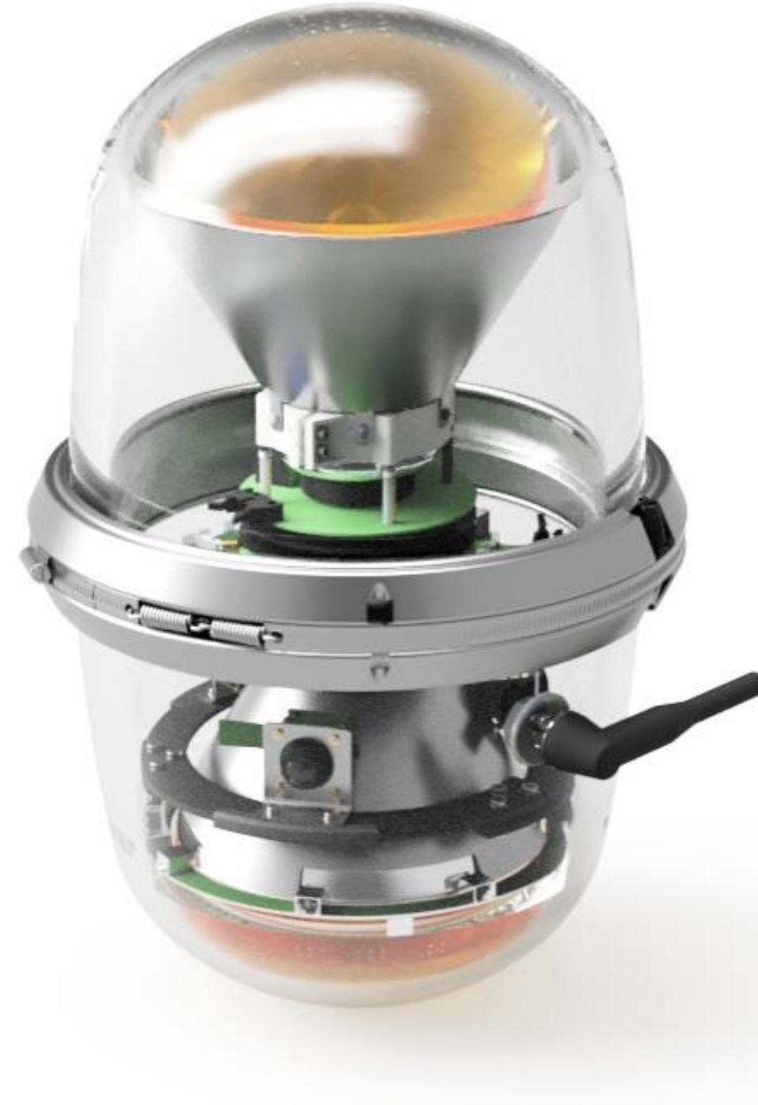
Ellipsoid glass with thin diameter with 2 PMT
