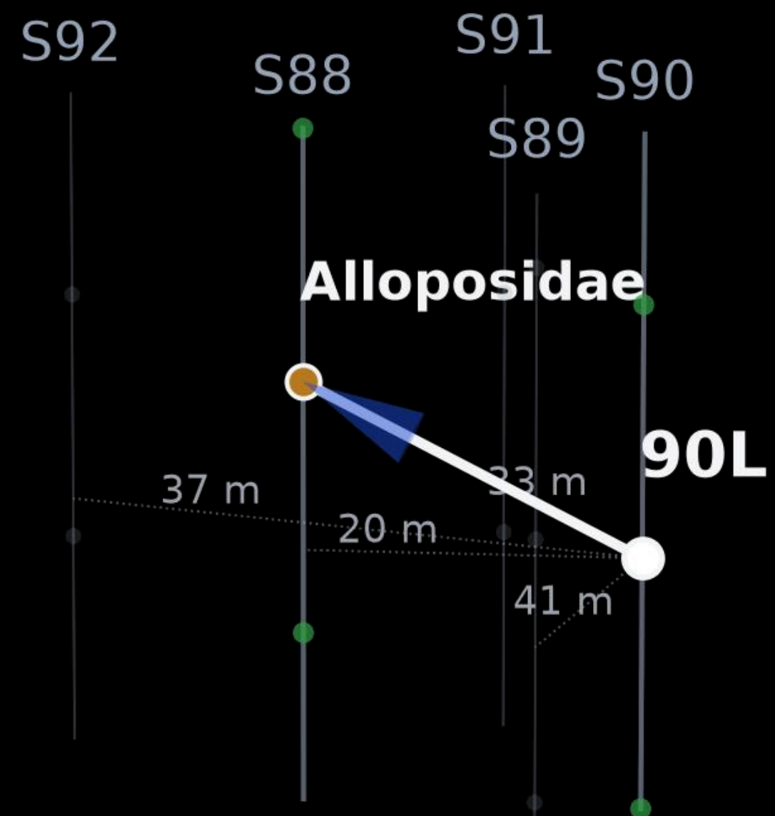
Camera 90L watching string 88 blue LED of ~10 mW in 20 m distance
