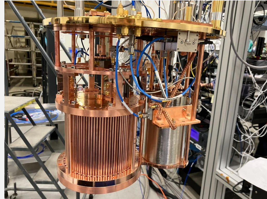
Cavity mounted inside ALPHA fridge
