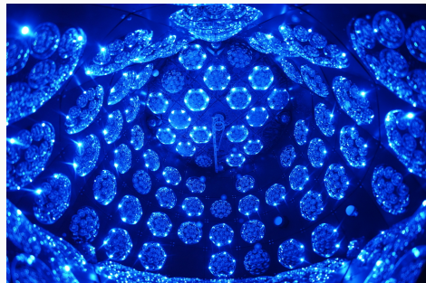
WCTE interior: multi-PMTs lit during operation.
