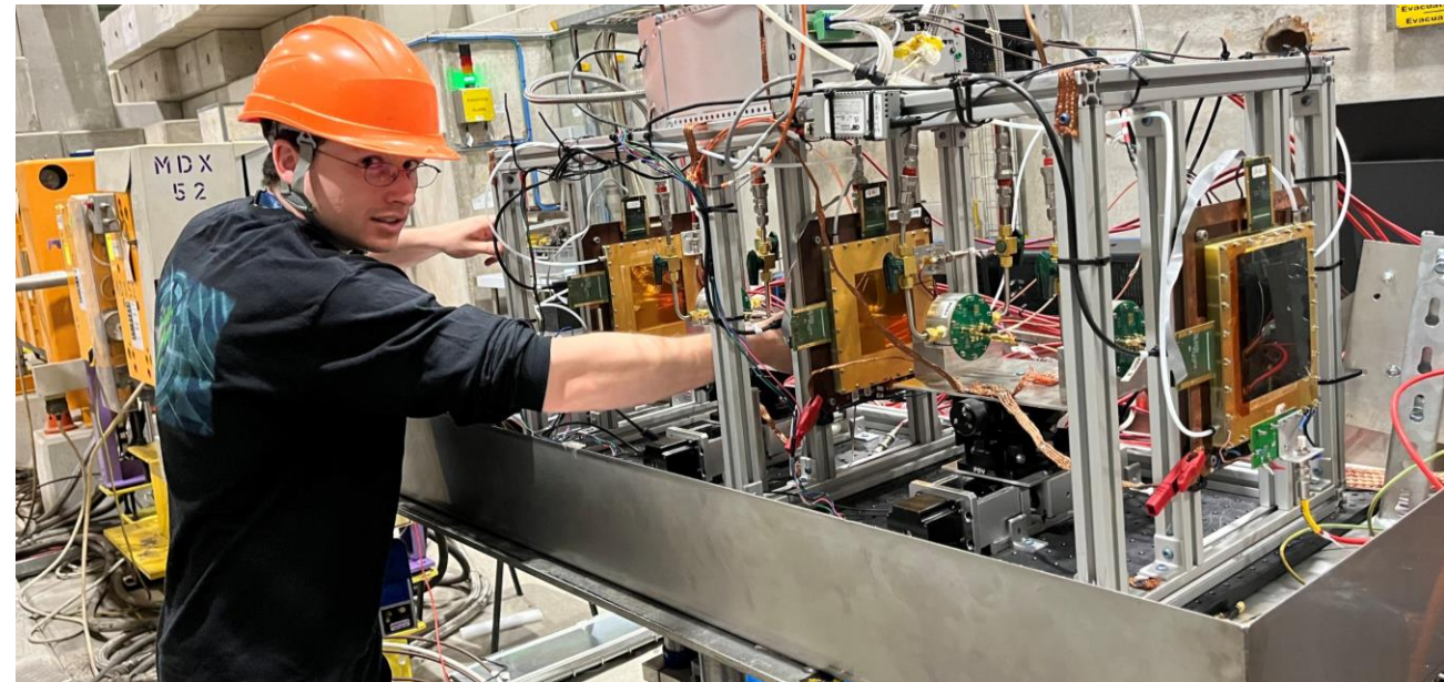
\mu RWELL-PICOSEC telescope used in 2024 beam test @ CERN
