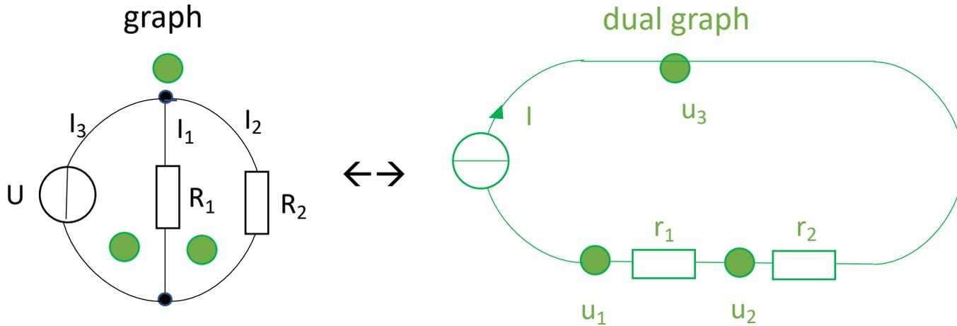
*converted parallel circuit into serial circuit*
