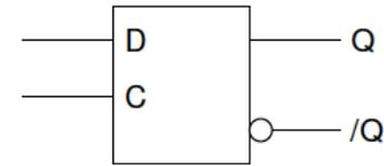
.... can be used to construct **serial shift register**
