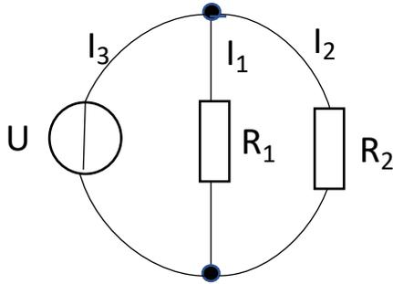
$$I_3 = -I_1 - I_2 = U \left( \frac{1}{R_1} + \frac{1}{R_2} \right)$$
