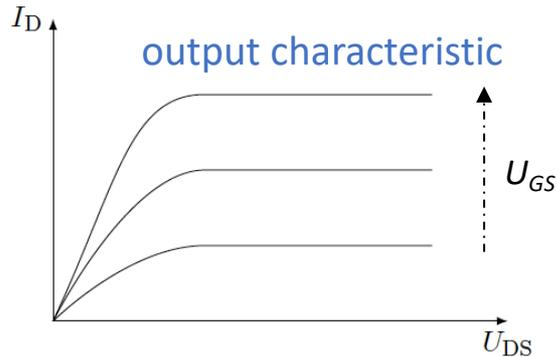
Typically, smaller transconductance than BJT (output current /input voltage)
