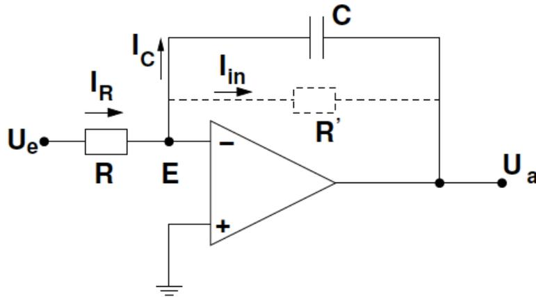
Virtual ground offset by input current
