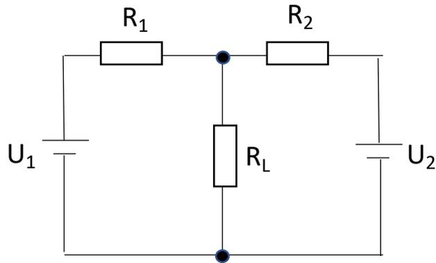
Step1: remove load and shorten sources. Then calculate total Thevenin resistance  $R_T$  wrt A/B
