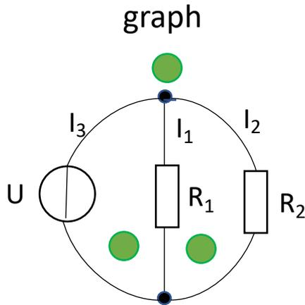
$$I_3 = -I_1 - I_2 = U \left( \frac{1}{R_1} + \frac{1}{R_2} \right)$$
