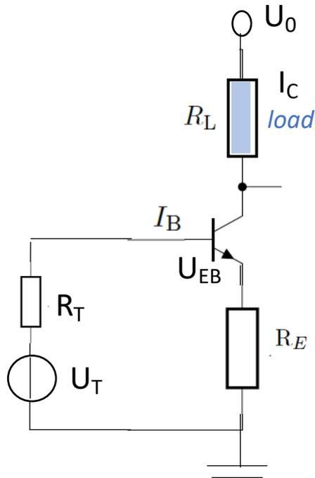
Reminder: We can stabilize the working point by adding an emitter resistance
