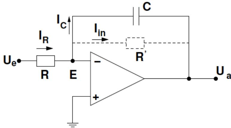
Virtual ground offset by input current
