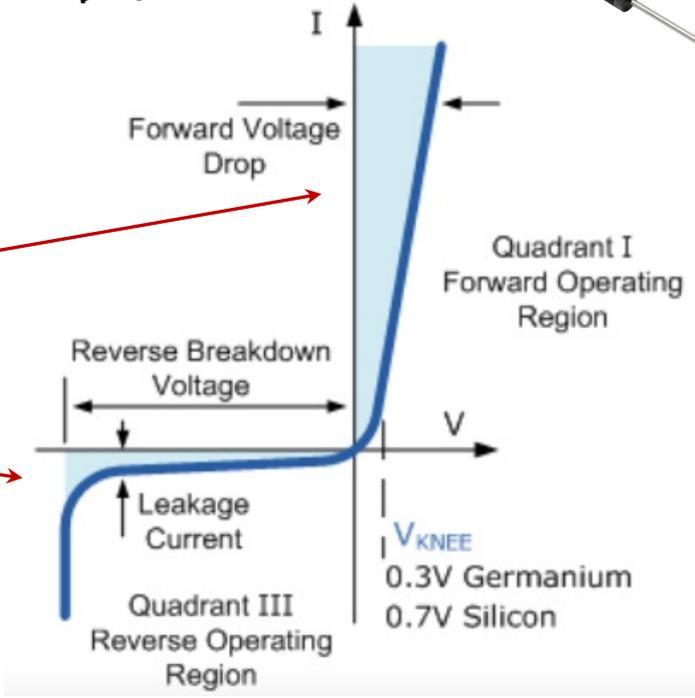
Electrons cross the junction from n to p type → depletion zone, barrier voltage
