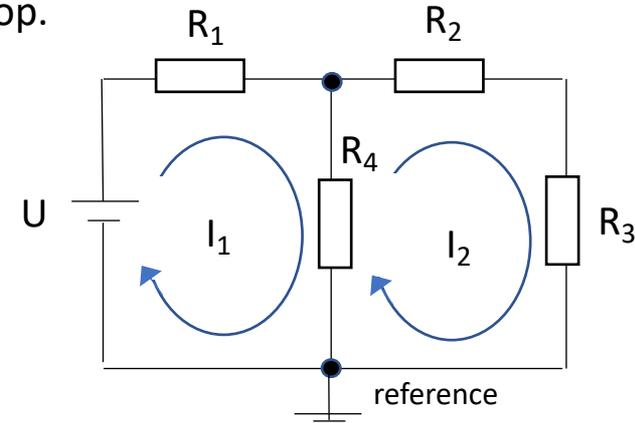
Example: Mesh 1:  $R_1 I_1 + R_4 (I_1 - I_2) = U$
