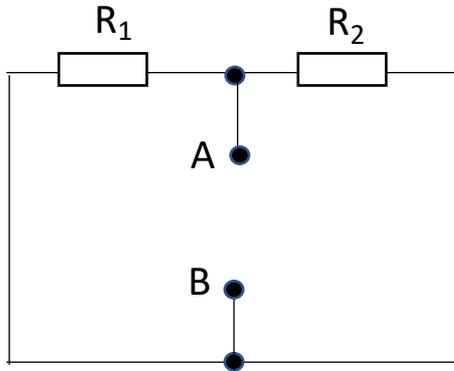
$$R_T = R_1 || R_2 = \frac{R_1 R_2}{R_1 + R_2}$$
