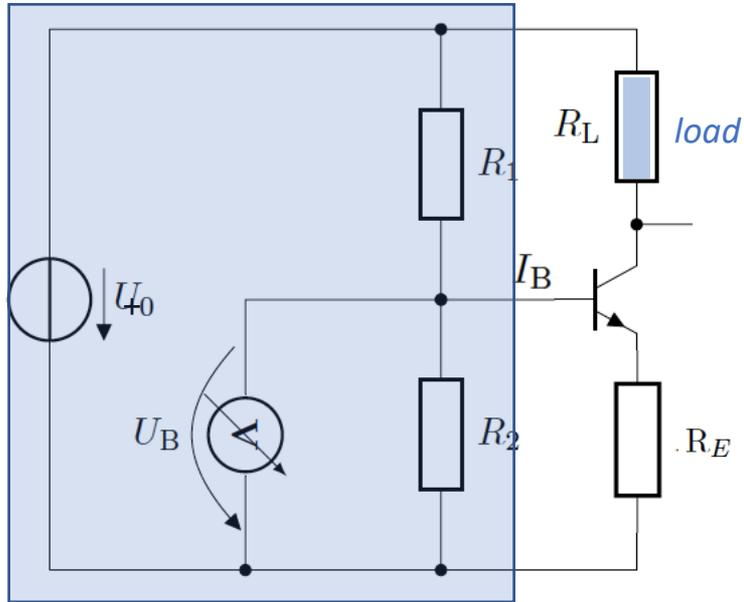
In order to simplify the calculations, we want to replace the voltage divider by the Thevenin equivalent
