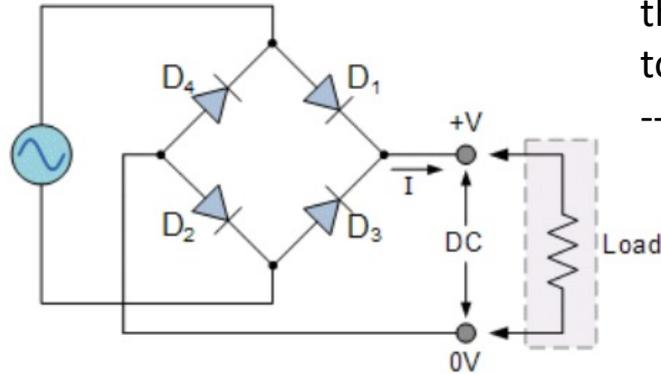
Diodes are arranged such that the positive pole is always connected to the same point.
