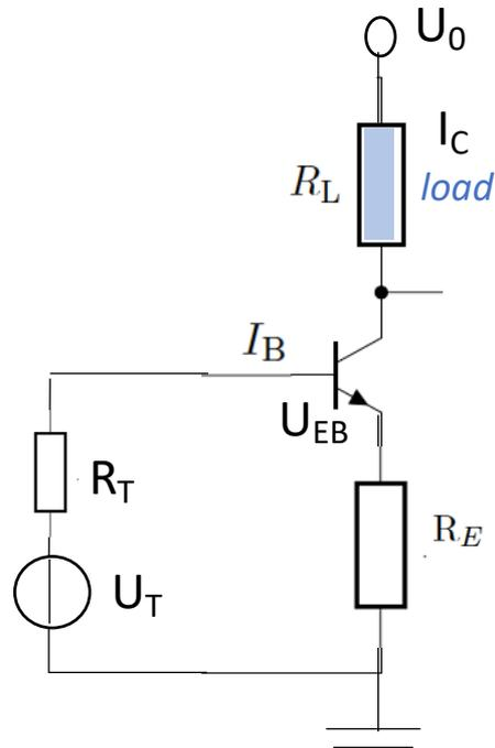
In order to simplify the calculations, we want to replace the voltage divider by the Thevenin equivalent
