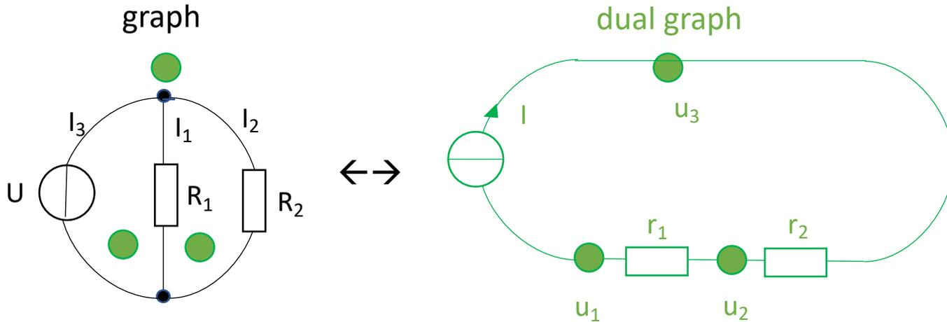
*converted parallel circuit into serial circuit*
