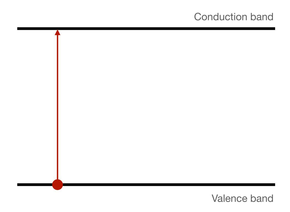
Charge carrier production in semiconductors relates to transitions from the valence to conduction band
