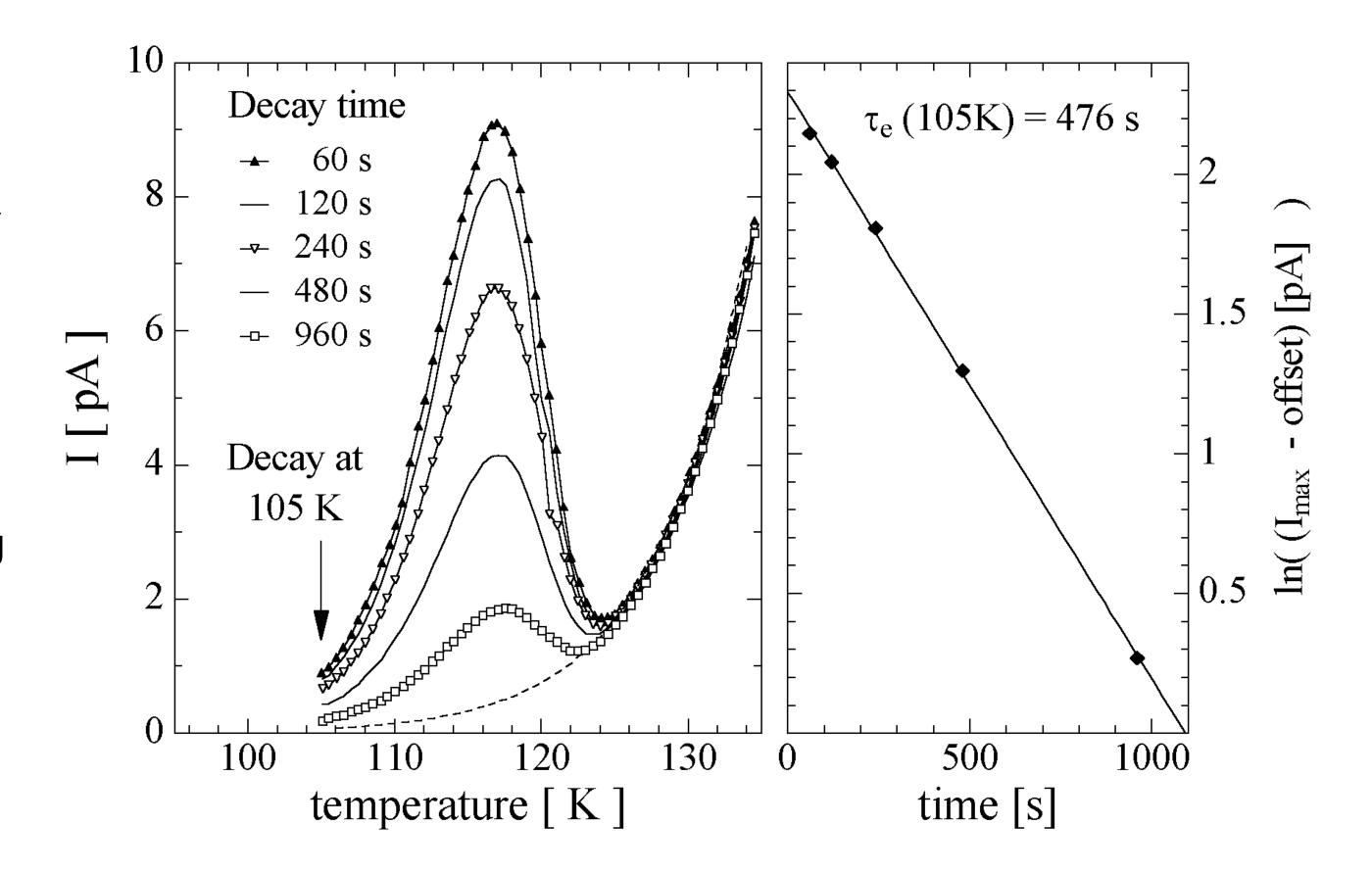
Depending on the charge and type of the defect (and bulk), the departure of a charge carrier may be affected by the resulting space charge
