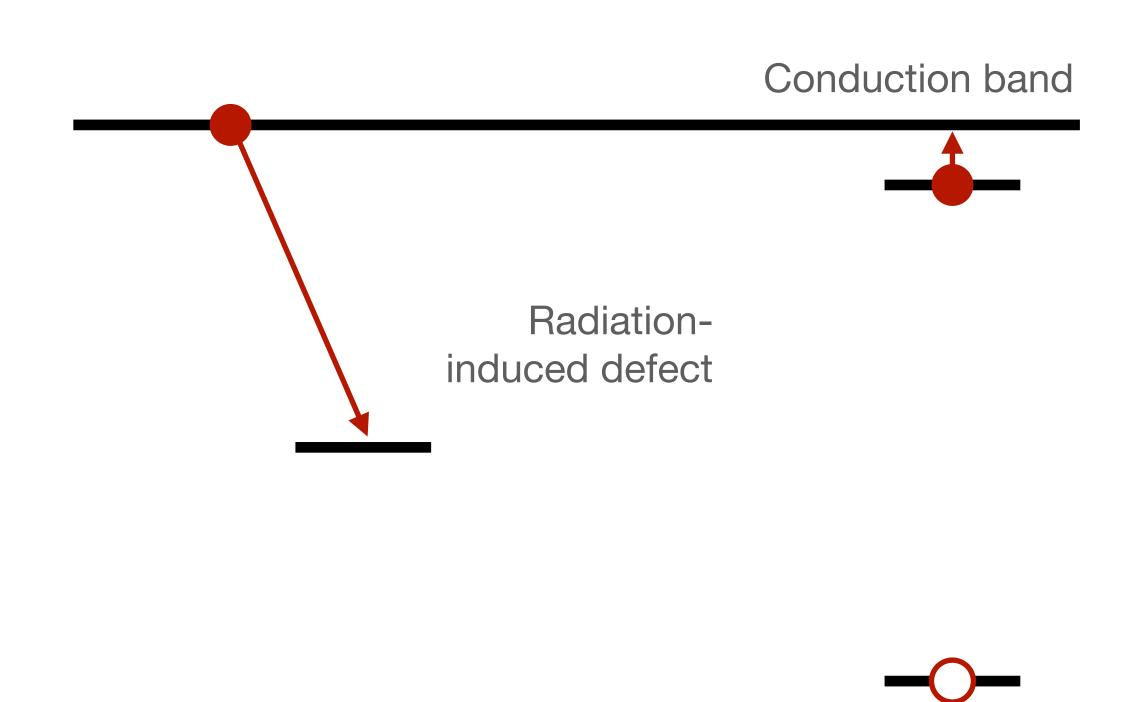
Charge carrier production in semiconductors relates to transitions from the valence to conduction band
