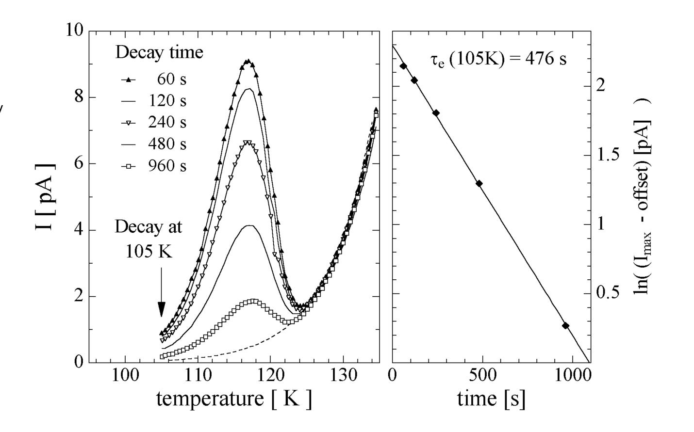
The peak temperature is not a terribly precise way to extract the activation energy of the traps - can instead perform measurements at different times and temperatures to extract true activation energy
