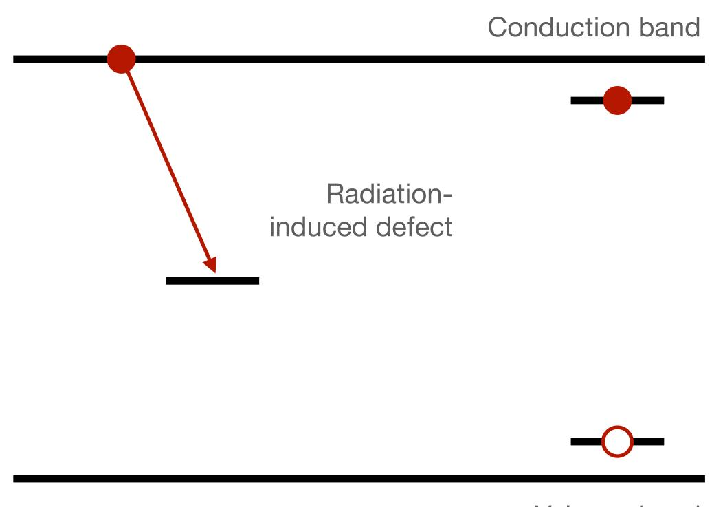
Charge carrier production in semiconductors relates to transitions from the valence to conduction band
