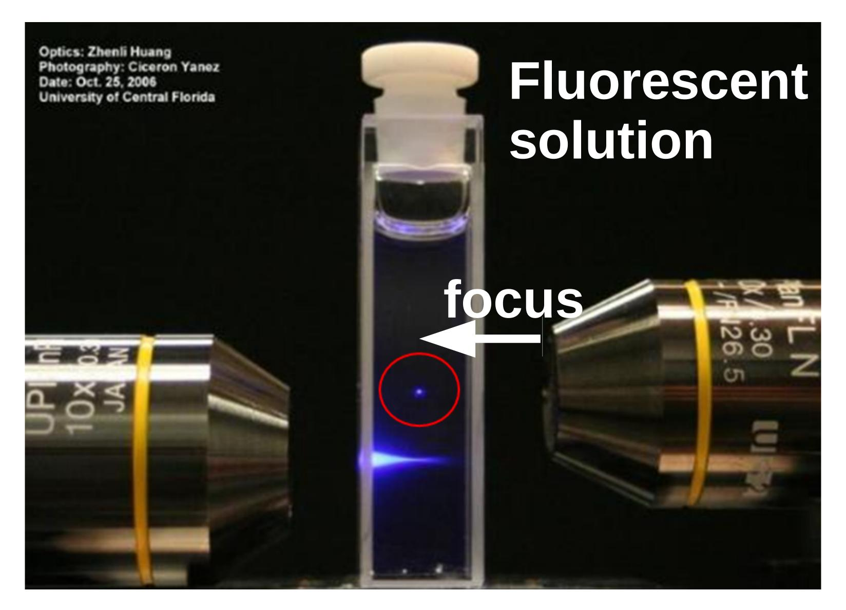
Lasers for TPA-TCT have to be sharply pulsed in order to generate enough photons at the focal point to lead to appreciable charge carrier generation
