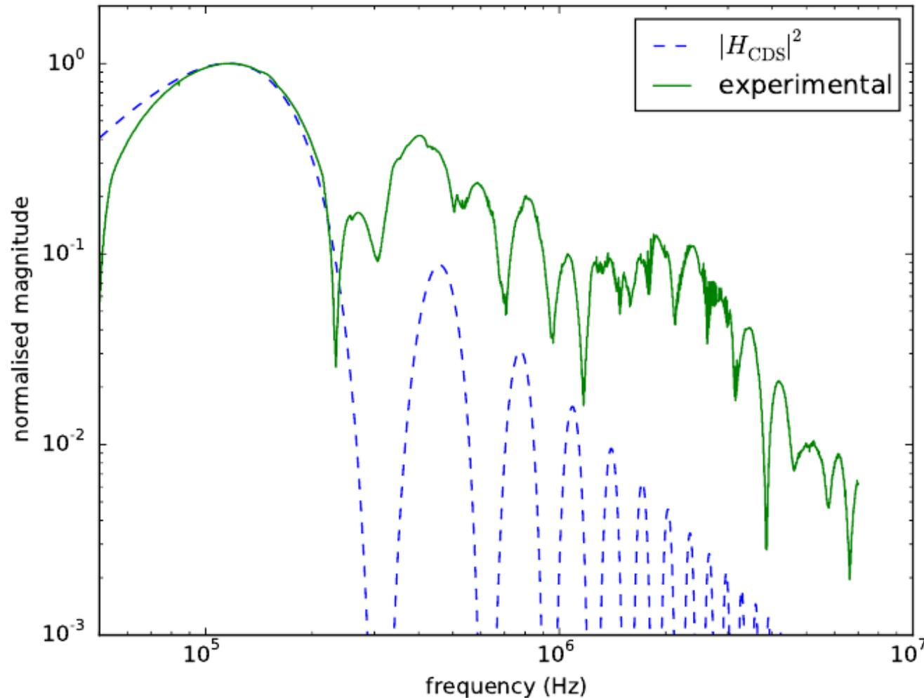
Measured on an e2v CCD261 during my PhD thesis days using a new technique I first developed (though it is pretty obvious how to do it)
