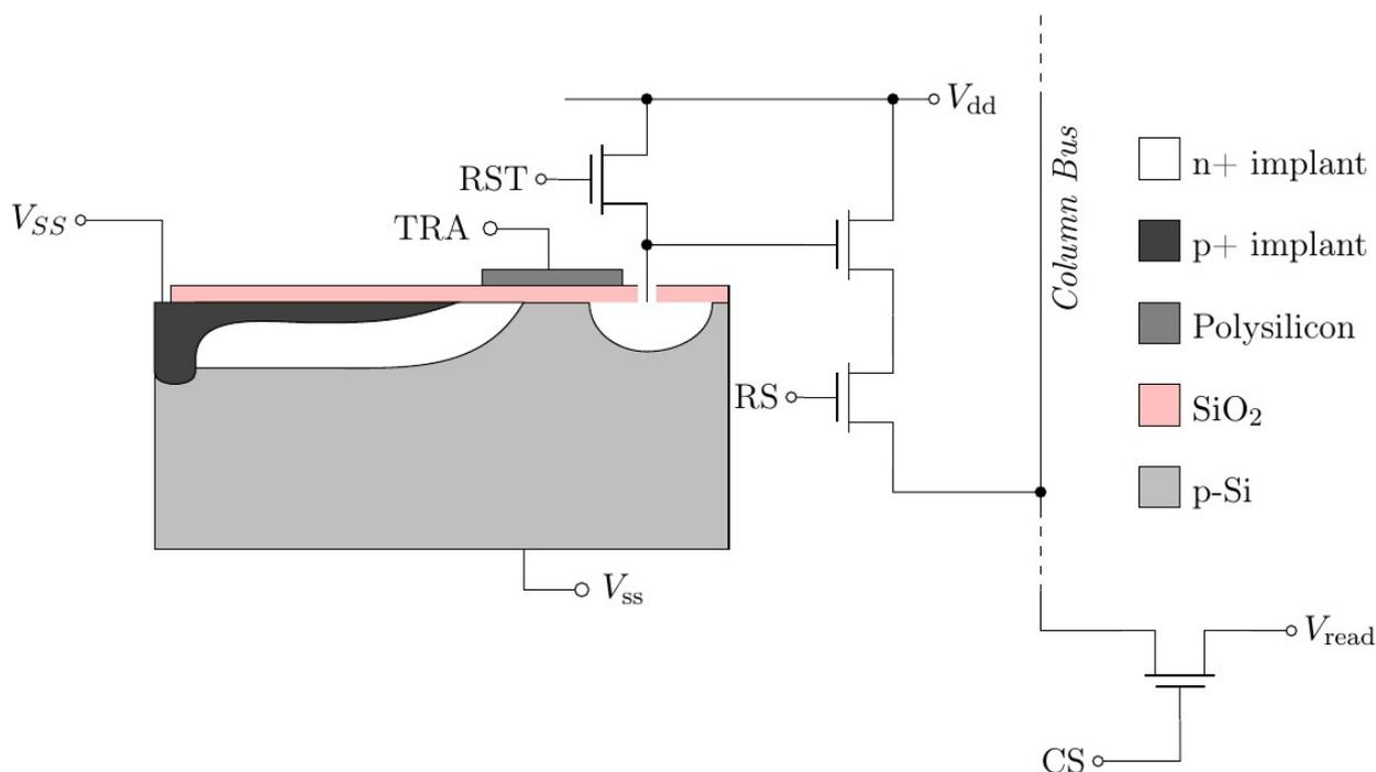
“Pinned” photodiode structure mimics buried channel construction of CCD (invented by E. Fossum in early 90s).
