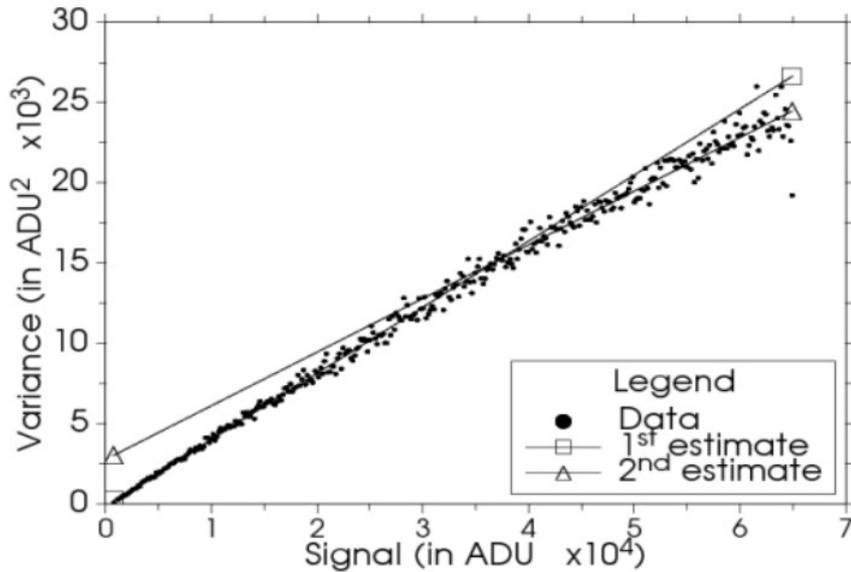
First observed (in 2006, left) by Mark Downing of ESO as an unexplained non-linearity in mean-variance data
