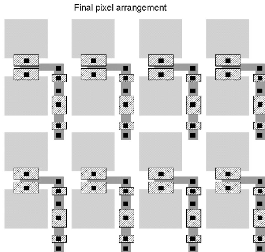
**Figure 1. Conventional two-shared pixel architecture. Unit cell (top) and final pixel arrangement (bottom).**
