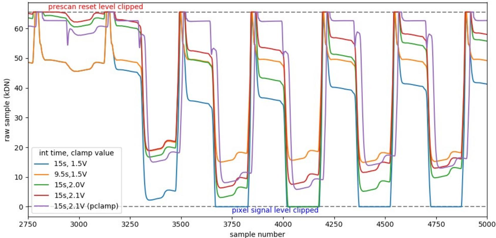
Digital CDS approximates the analog CDS by oversampling. It has its own problems (in particular ADC clipping!), but is (surprisingly) generally less temperamental than analog CDS.
