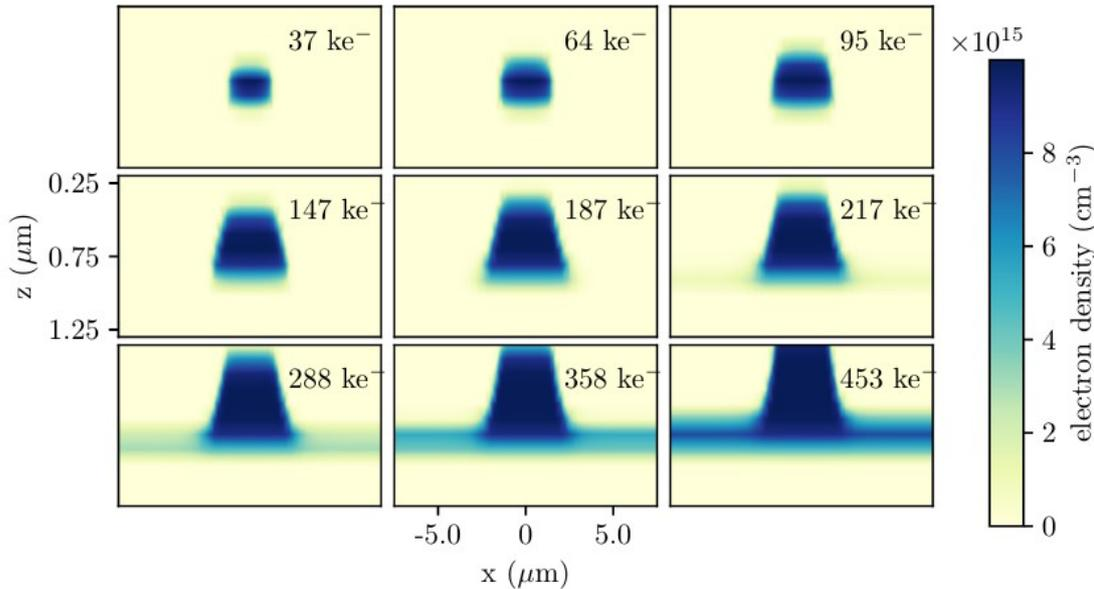
Photons absorbed in the volume, and then collected by strong drift field until they reach the storage “well”.
