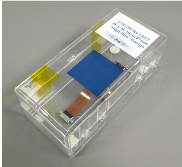
**Left:** a truly “boutique” level AR coating as used for astronomical instrumentation gives detector a very blue colour (longer wavelengths absorbed very efficiently and reflectivity attenuated)
