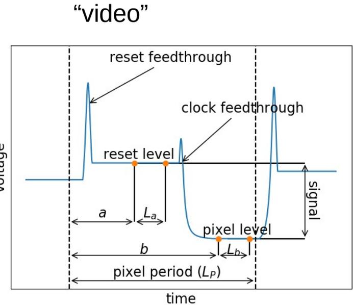
The typical CCD readout circuit is simply a node capacitance with a source follower. There is also a (usually MOSFET) transistor to reset the node to “empty”.
