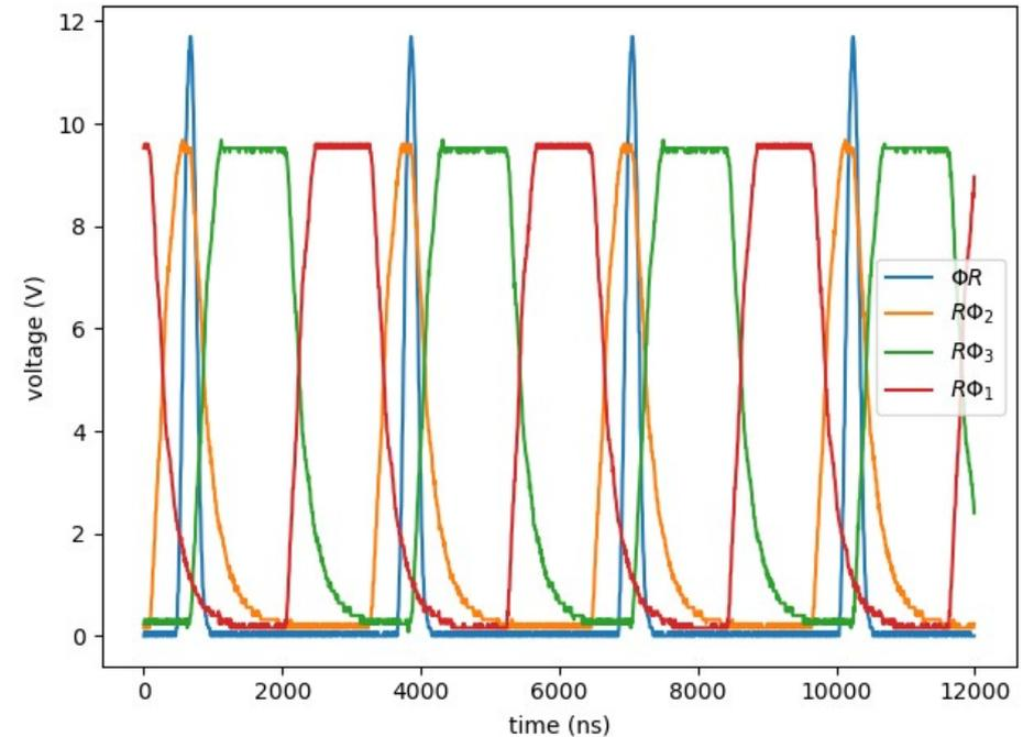
In OPMD we have a very high speed state of the art digital readout which oversamples the CCD clocks hugely (each channel runs at **100MHZ!!!**). This is fine for 16 channels of one sensor, but for ~3000 video channels in LSST camera would be impractical due to power & cooling requirements.
