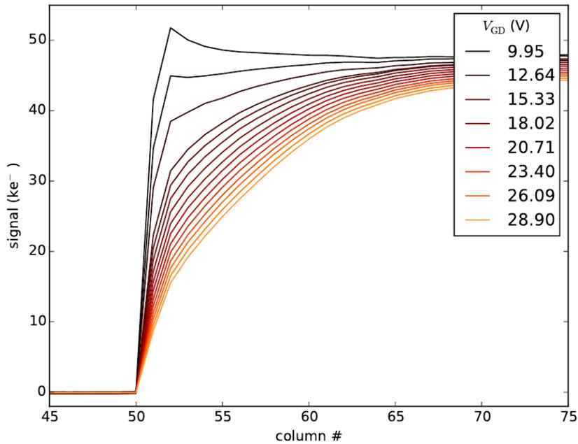
The guard drain / “scupper” field at the edge of the sensor “drags” incident charge around, which causes a shift in position of measured sources. This can be seen in both flat field measurements (left, Weatherill 2016) and in spot projection measurements (below, due to Bradshaw et al 2019).
