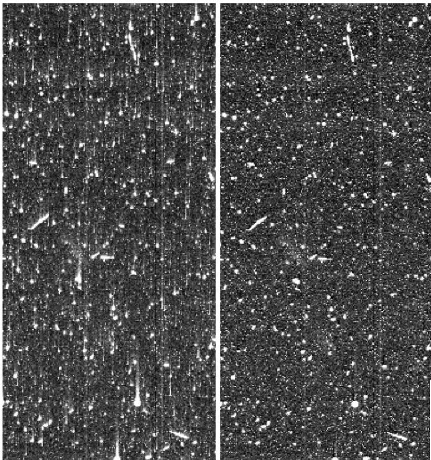
In brief – they aren't. Particularly susceptible to displacement damage which causes increased CTI(**left**) after a tiny (in particle physics terms) amount of radiation (mission lifetime dose of Euclid is something like  $\sim 10^{10}$  protons  $\text{cm}^{-2}$ ).
