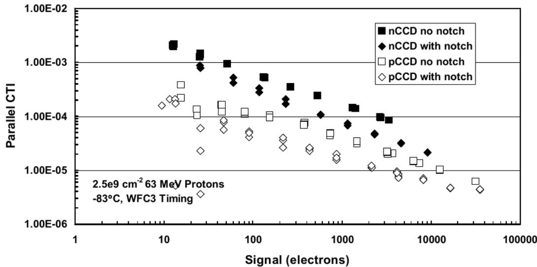
Build CCD on p-type substrate (n-type buried channel), it now collects holes rather than electrons.
