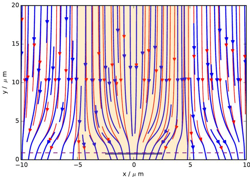
Upper left: nice visualisation of pixel boundaries from BFE simulation courtesy of Antiloqus et al (2014)
