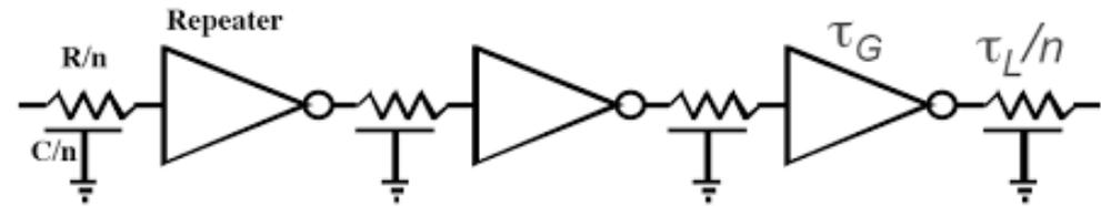
A long interconnect line  $L$  is broken into  $n$  segments
