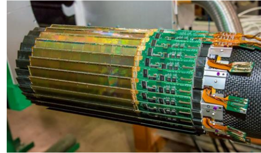
The vertex detector of the STAR experiment, the first to use CMOS MAPS
