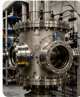
Example: FELIX-LISA end-station for THz/F-IR irradiation and in-situ measurements.
