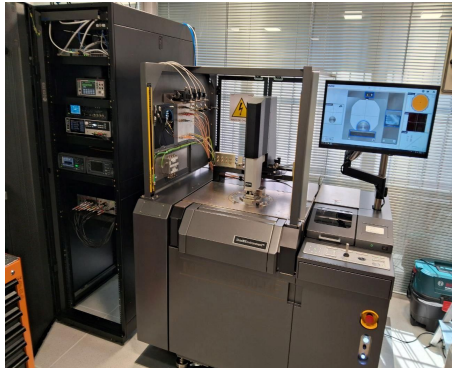
Probe Station setup at USP
