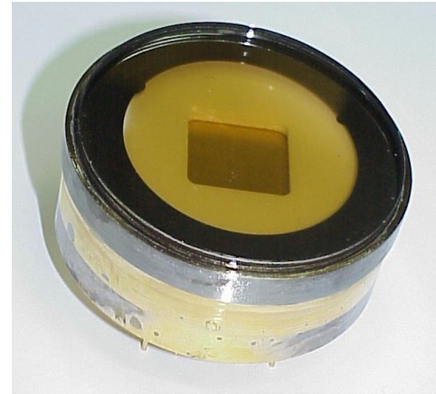
GEM with semi-transparent Photocathode (K-Cs-Sb)
