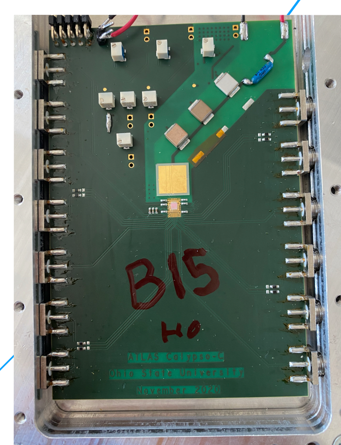
Detector module box with a 10 \times 10 \text{ mm}^2 pCVD diamond and Calypso FE ver. C.
