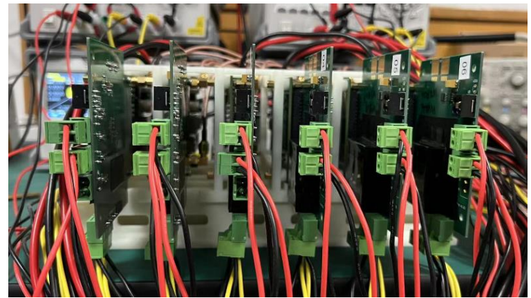
Telescope made by TaichuPix3
