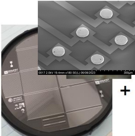
Pad wafer with 6 full chain dies
