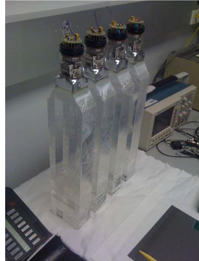
This is a preassembly photo of the energy detector before wrapping and placing them stacked inside the metal housing.
