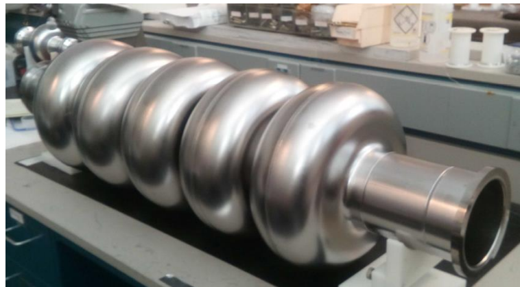
800 MHz bulk Nb 5-cell cavity Prototype fulfilling FCC specs JLAB, F. Marhauser
