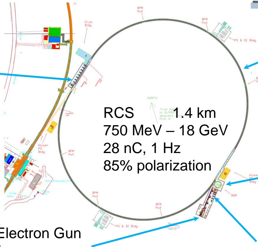
S-band linac, 750 MeV, 30 Hz, 1 nC single bunch
