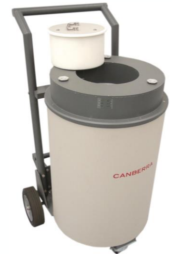
Active Well Coincidence Counter based on 48 ^3\text{He} tubes [3].
