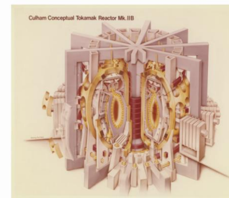
A Tokamak Design from 1975. Credit Unknown, Courtesy IAEA Archives
