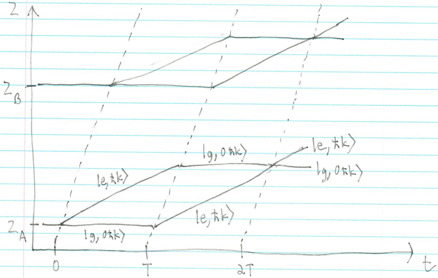
The laser, with frequency  $\omega$ , is pulsed on at times  $0, T$ , and  $2T$ . The two interferometers start at slightly different times due to the finite speed of light as it travels across the baseline. The dashed lines show the photon trajectories, with  $c$  exaggerated as unrealistically small for ease of visualization.
