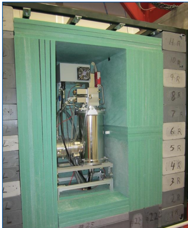
2.5 MeV D-D neutron generator
