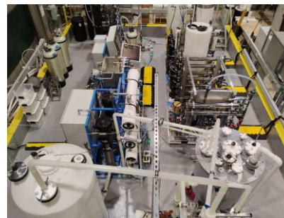
30-ton testbed for future liquid calorimetry
