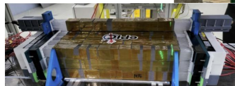
Pb/SciFi test article built by BIC S. Korea team
