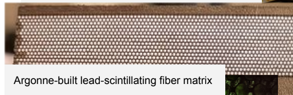
Pb/SciFi test article built by BIC S. Korea team
