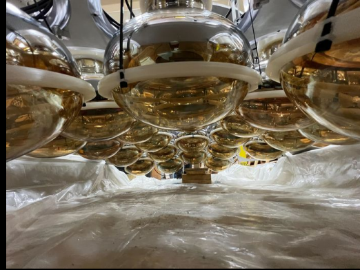
First PMTs installed (Oct. 2023)
