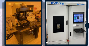
Chromium deposition & lift-off
