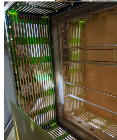
Iceberg TPC (~1m 3 ): wires planes in the middle, 2 drift volumes
