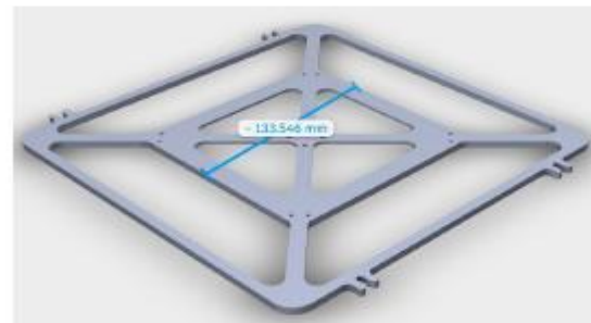
Window support used during assembly
