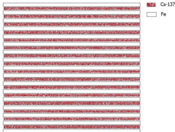
Volume source representing the activated slab for validation of MCNP6.1 models (VisedX_24E)
