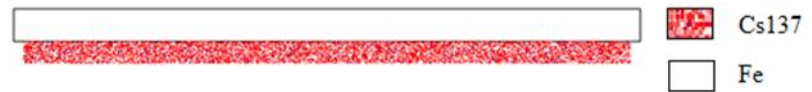
Volume source representing the surface contamination on a slab for validation of MCNP6.1 models (VisedX_24E)
