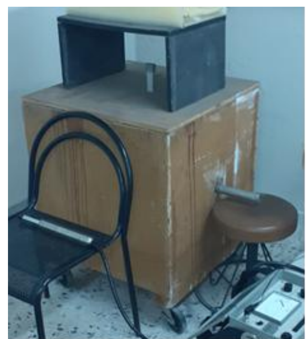
Fig. 2: Paraffin pile: H = 0.63 m, W = 0.63 m, D = 0.63 m
