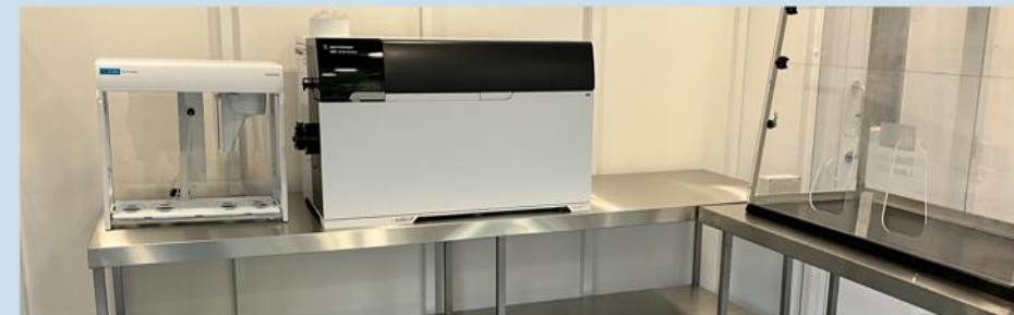
ICP-MS (Surface): Newly installed system for trace element analysis and isotopic ratio measurements.
