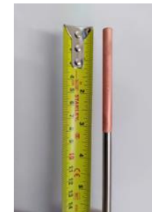
Copper electroforming at Boulby
