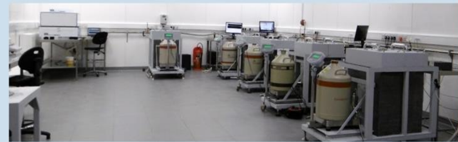
BUGS (UG): A range of HPGe detectors and alpha particle detectors for intrinsic and surface radioactivity measurements.
