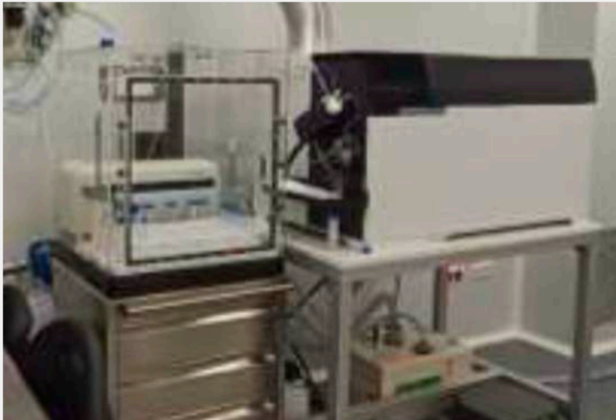
ICPMS-QQQ underground 2 ppq sensitivity in Uranium
