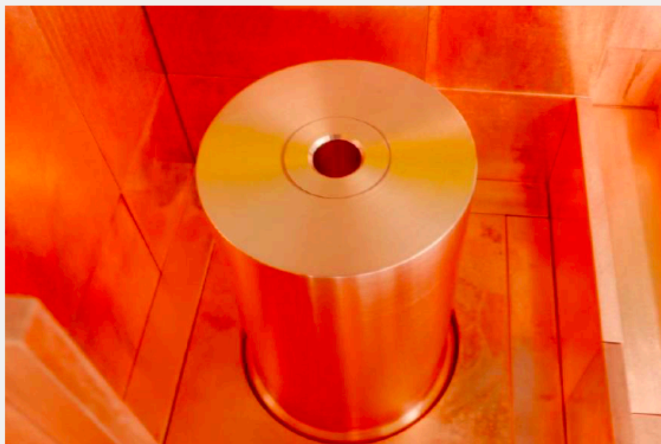
HPGe detector GeRysy \mu\text{Bq/kg} sensitivity
