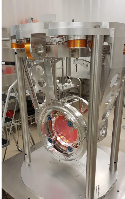
Mirrors weight 42 kg to reduce the radiation pressure noise
