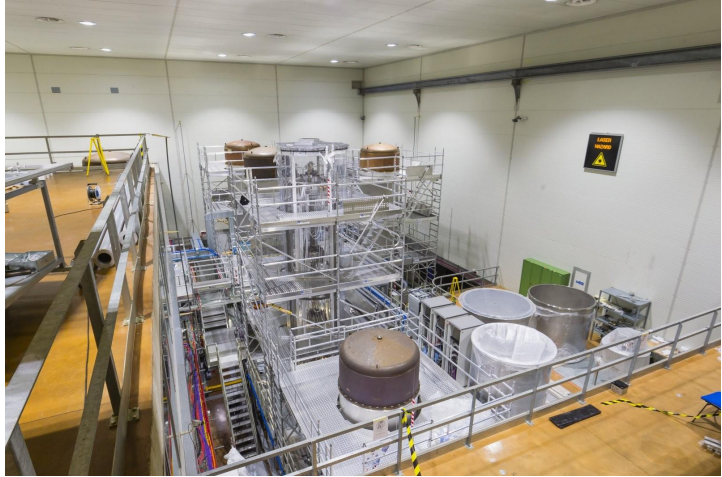
Superattenuators for seismic isolation
